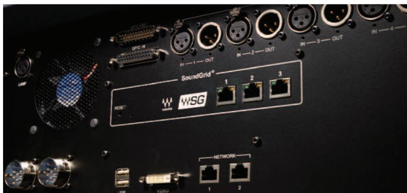
An integrated, preconfigured 64-by-64 Waves interface enables direct multitrack recording to a companion laptop, plus connection to a Waves MultiRack SoundGrid server for operator access via the left-hand touch screen to Waves-brand plug-ins running on the SoundGrid server.
